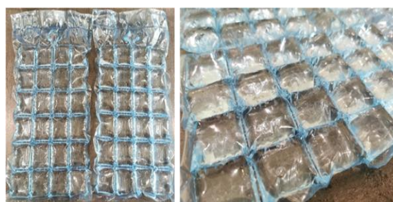
Figure 1. The synthesised PCMs packed in bubble wrap.
