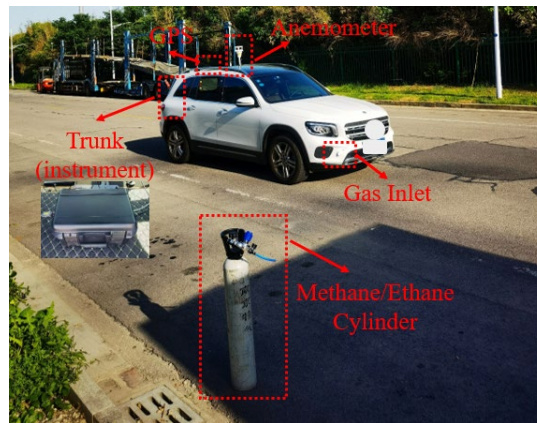
Figure 6. Field test of monitoring CH 4 /C 2 H 6 cylinder leakage at Zhenwu Road, Southeast University Science Park.
