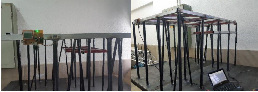
Figure 5. Laboratory model of the pile-deck wharf and instrumentation layout for experimental modal analysis.
