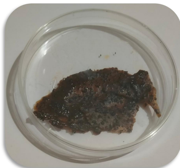
Figure 5. Image of biocomposite film synthesized from solid residue collected post extract of fruit peels of M. balbisiana var elavazhai .
