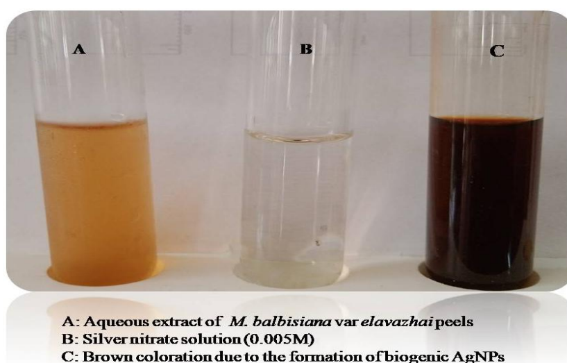
Figure 1. a, Musa balbisiana var elavazhai peel aqueous extract; b, 0.005M silver nitrate ( \text{AgNO}_3 ) solution; c, Dark reddish-brown solution indicating the formation of silver nanoparticles.
