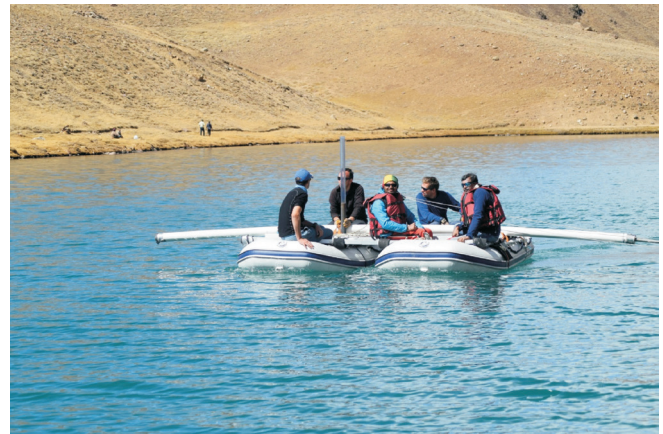
Figure 4: Returning to shore at lake Chandra Tal after retrieving one of the long piston cores. The raft is mounted on top of two light weight rubber boats with a small outboard engine in the back.
